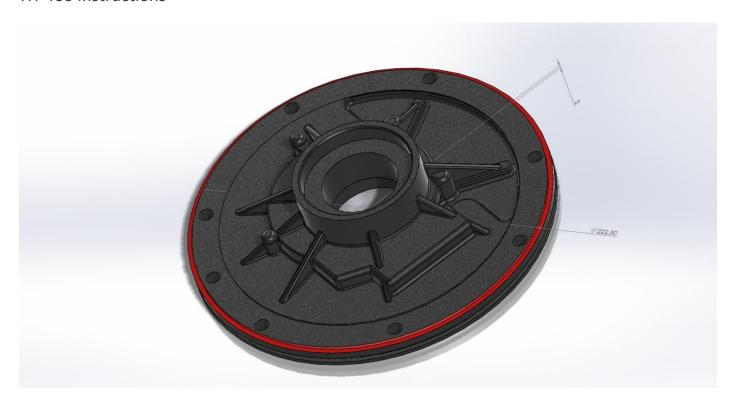
As the TH-400 pump does not have an accurate lip to locate the bell housing on, the pump has to be machined down to a diameter of 222.5mm x 2mm deep. This gives the Dellow Conversions bell housing a definitive locating point.
